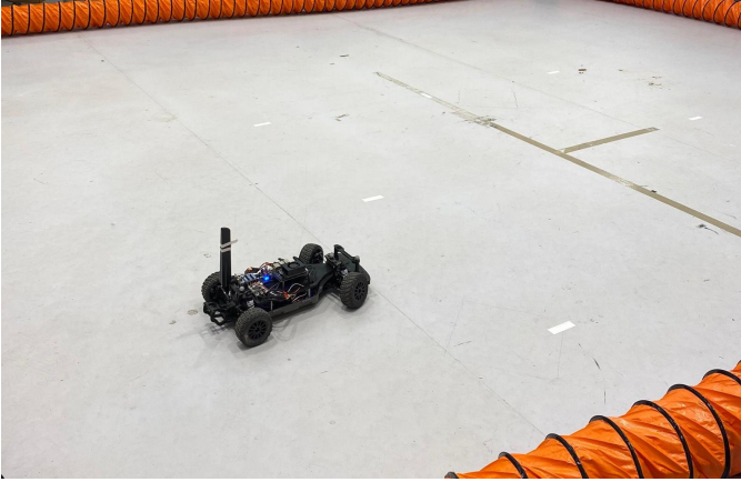
Fig. 1. Experimental setup on the custom indoor circuit. The F1TENTH vehicle is shown navigating within the track boundaries defined by flexible orange tubing, utilizing the Vicon motion capture system for real-time state estimation and MPCC controller with ROS2.
